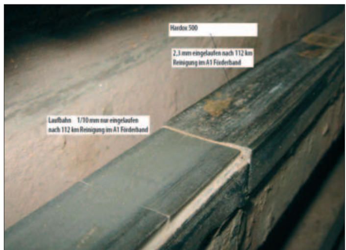
Fig. 8: Comparison between edges made of tungsten carbide and Hardox 500
