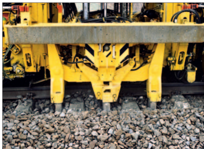
Fig. 4: Centre-tool two-sleeper tamping unit on an operating 09-32 CSM
