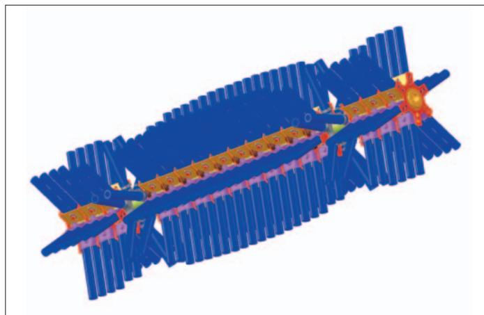
Fig. 4: New brush elements for ballast distributing and profiling machine
