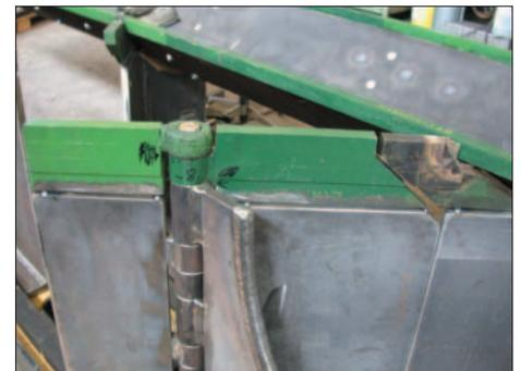
Fig. 5: Hardened metal wearing edge for ballast ploughs
