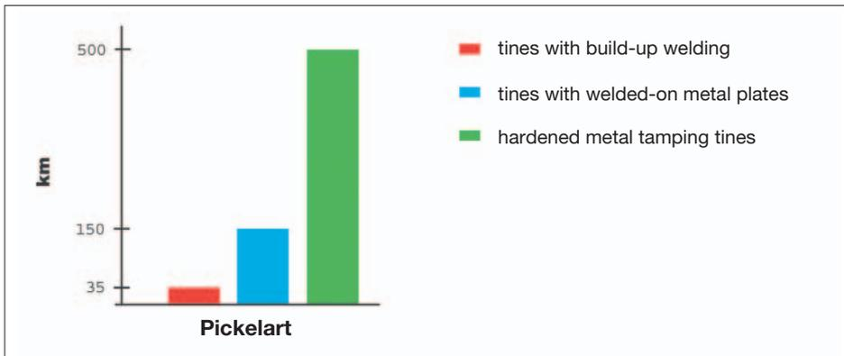
Fig. 3: Comparison of the service life of various types of tamping tines
