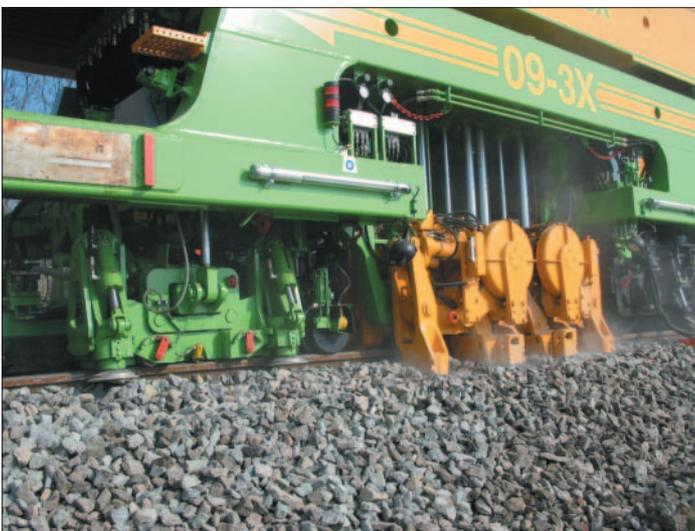
Fig. 1: Tamping unit of 09-3X Tamping Express
