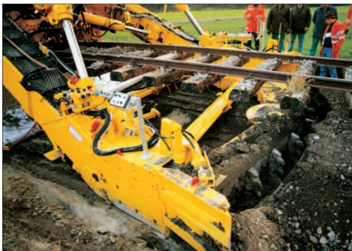
Fig. 6: Excavating chain of a formation rehabilitation machine
