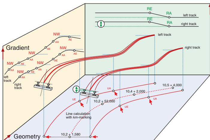
Fig 1. The Deutsche Bahn Reference System provides a three-dimensional representation of the track position.
