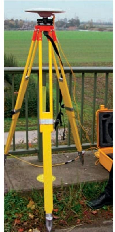
A GPS reference station provides the connection to SurVer.
