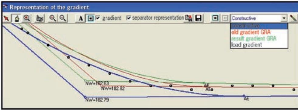
Fig 2. ATREK provides automatic gradient calculation with interactive processing functions.
