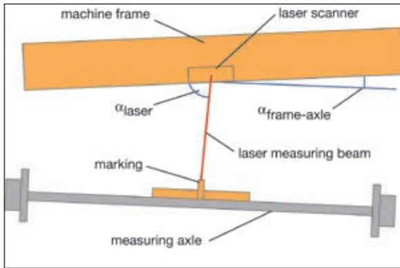
Fig 5. The functioning of the laser compensation scanner.
