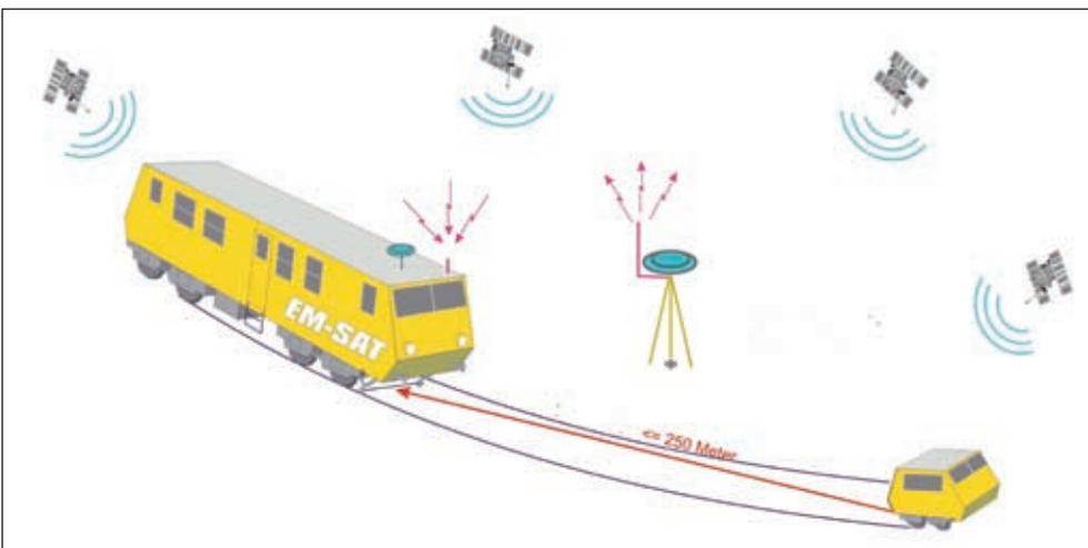
GNBAHN/PM runs on a pen-top calculator which is connected to the gauge-centred rolling surveying system carrier known as SurVer.
