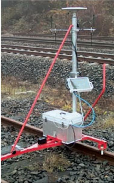
established with a geometric accuracy of around  $\pm 10$  mm and a longitudinal level accuracy of around  $\pm 12$  mm. The actual track geometry in terms of level and line is then established in relation to the laser reference chord. Differential satellite measurements are recorded continuously at the same time.
