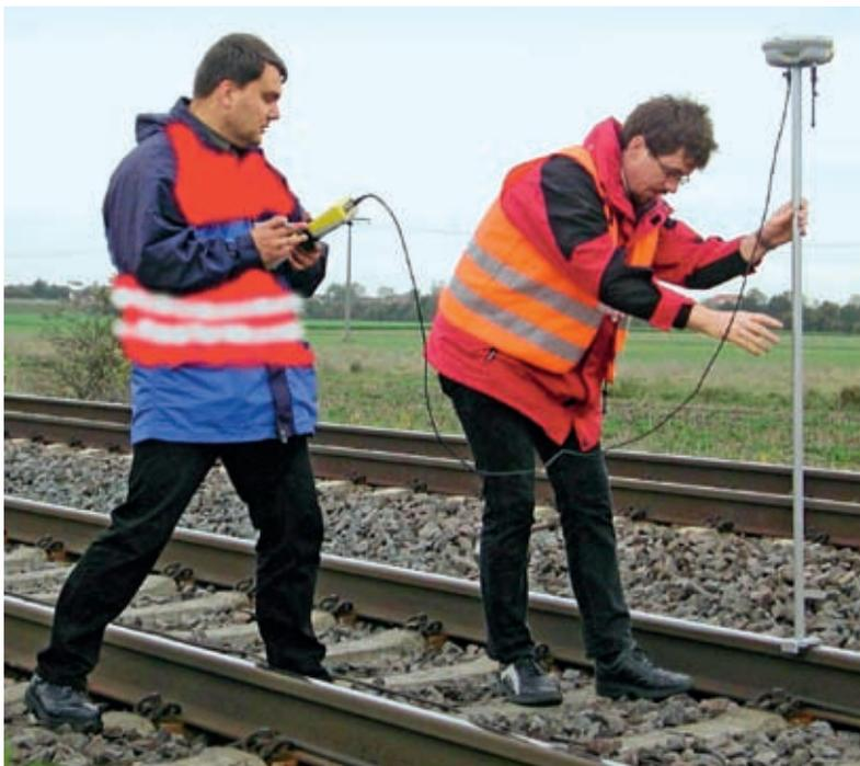
A satellite rod antenna can be used to undertake measurements individually on smaller worksites or when EM-SAT is not available.
