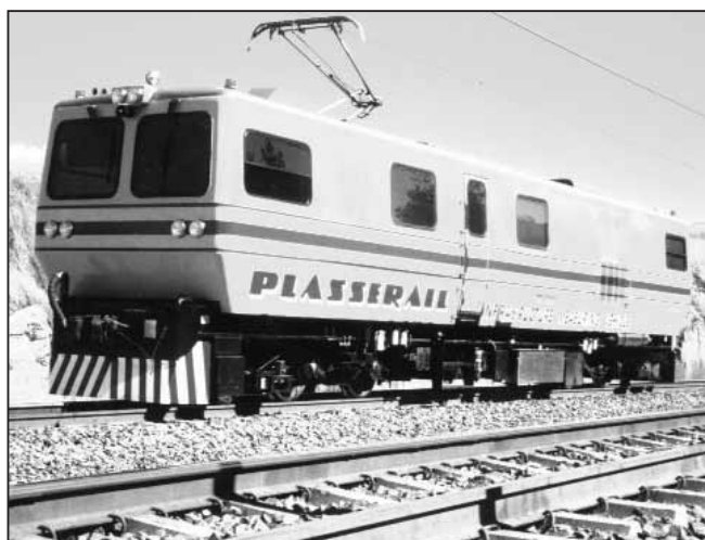
Fig. 1: IM2000 Infrastructure Measuring Car
