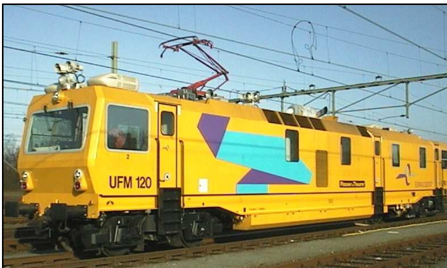
The UFM-120 track geometry car owned and operated by Eurailscout.
