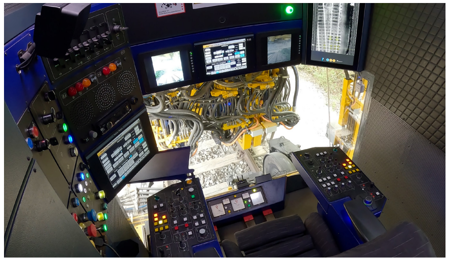
Autonomous tamping of a turnout without machine operators in the work cab during a demonstration at the iaf 2025.
