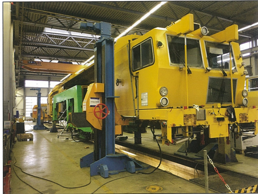
Fig. 2: The Unimat 09-16/4S with trailer. At the time this picture was taken, the progress made in maintaining and modernising the machine that was involved in a collision was very obvious
