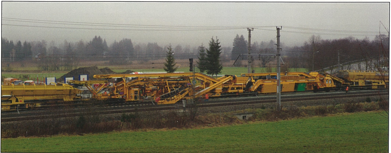
Fig. 1: The Plasser & Theurer URM 700 universal ballast bed cleaning machine for plain track and turnouts – this multi-talented machine can perform non-stop mechanised maintenance of turnouts, without requiring any dismantling of the turnout or digging of an access hole
