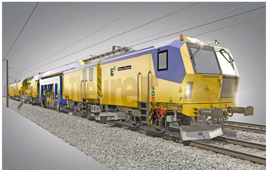
1: The new Unimat 09-8x4/4S BR Dynamic E 3 is a single machine that combines ballasting, tamping, profiling, stabilising, surveying, and post-measuring
