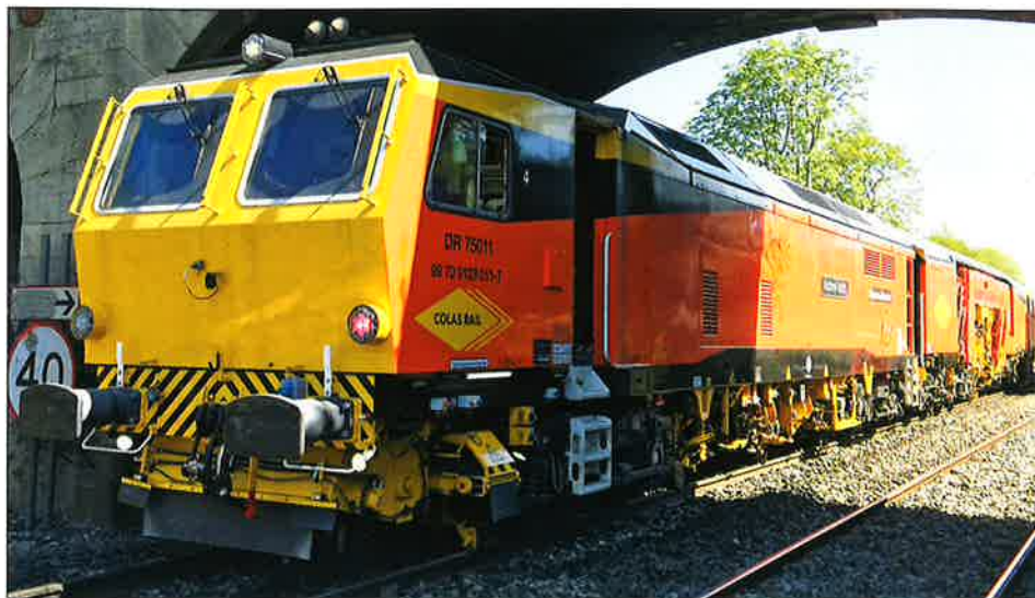
Above: Figure 1a - The Plasser & Theurer Unimat 09-4x4/4S Dynamic tamper.
