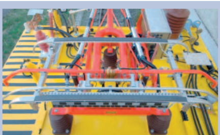
Fig. 3: Roof superstructure including the measurement electronics
