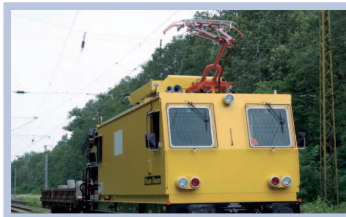
Fig. 6: Acceptance measurement of an overhead wire during a real-case deployment on Deutsch Bahn's network
