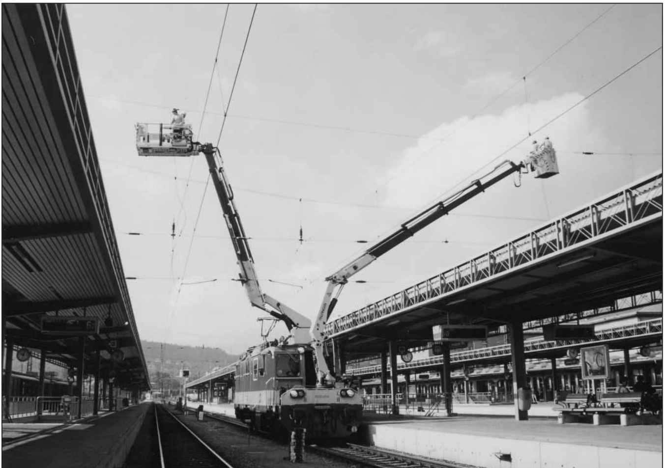
Fig. 5: Plasser & Theurer MTW 100.013/2 Motor Tower Car for catenary installation and maintenance, with freely moving elevating work platform and loading crane featuring work basket
