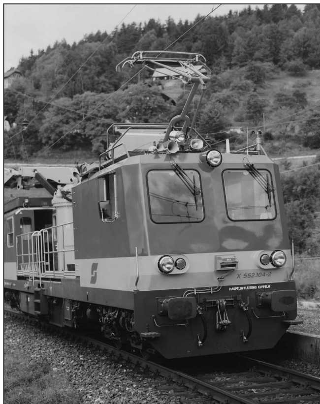
Fig. 8: Laser scanner (between the headlights) on the MTW 100.064/3 Motor Tower Car for catenary maintenance
