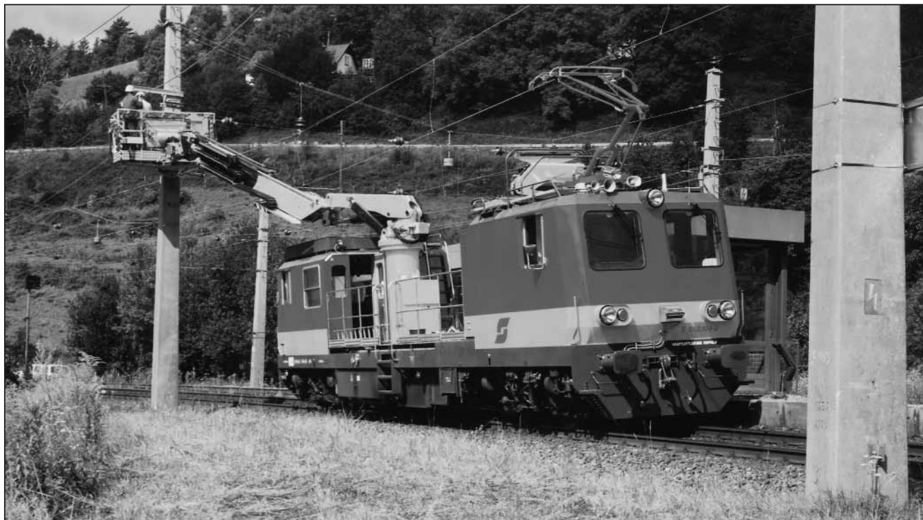
Fig. 2: Plasser & Theurer MTW 100.064/3 Motor Tower Car for catenary maintenance
