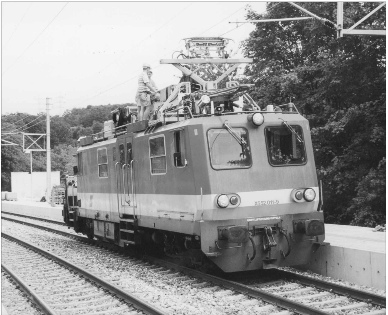
Fig. 3: Plasser & Theurer MTW 100.013/2 Motor Tower Car for catenary installation and maintenance
