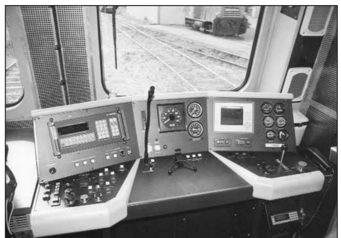
Fig. 4: Driver's desk with operating controls and display
